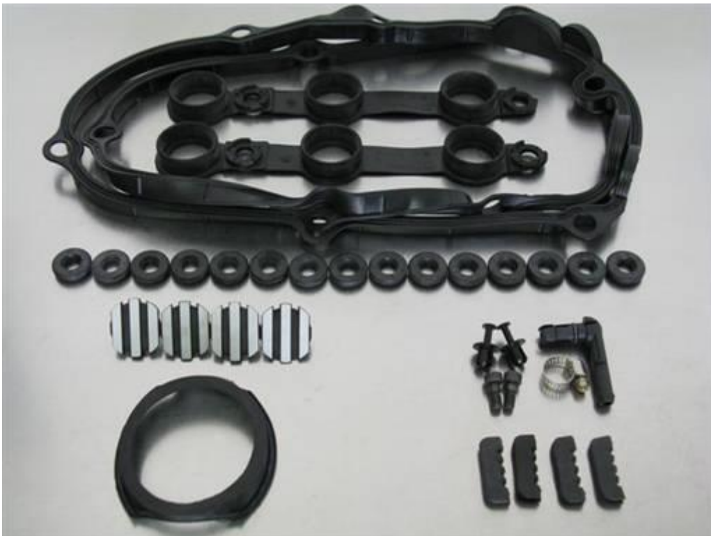
Double vanos seals repair kit (6-cyl) (BS001) $60/each ( www.beisansystems.com ), vanos gasket (11-36-1-433-817) 6.73/each, 2 x vanos oil hose/pipe washer (32-41-1-093-596) $.25/each
