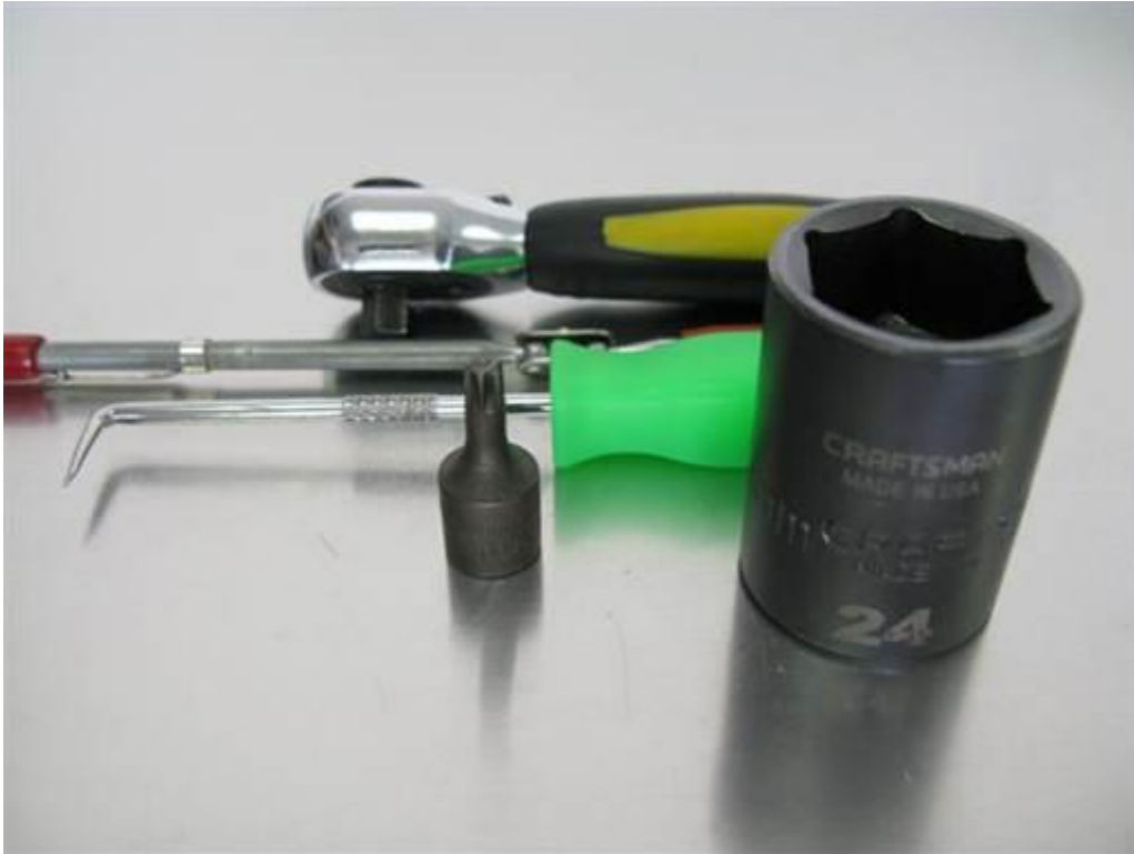
24mm impact socket 1/2", T30 torx bit socket 1/4", 90 degree pick tool, magnet pickup, 1/4" ratchet
