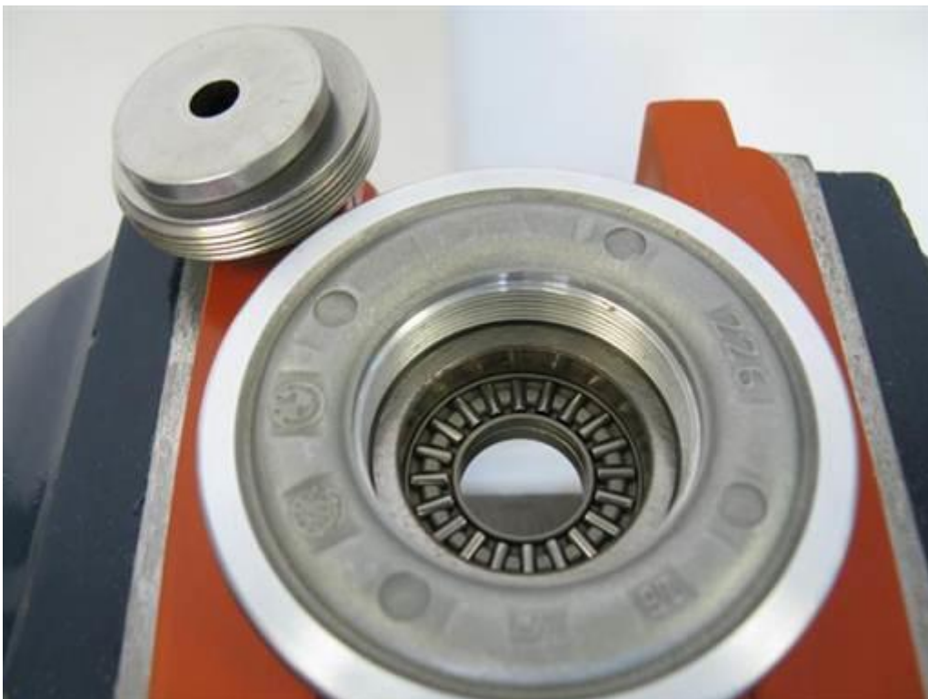
Remove bearing center washer (magnet pickup).
