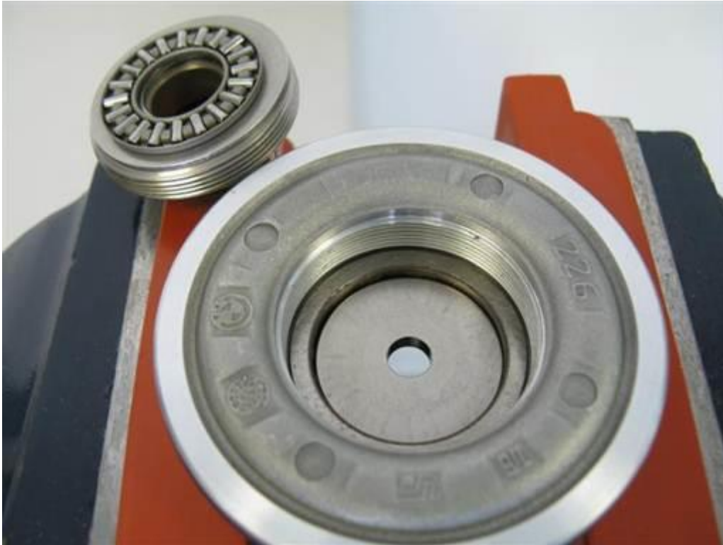
Remove bearing top thrust (roller) bearing (magnet pickup).
