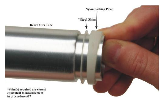
22. After re-seating the tube in the block the lock ring groove should now be exposed with no slop. Push spiral lock ring forward into grove locking tube in place.
