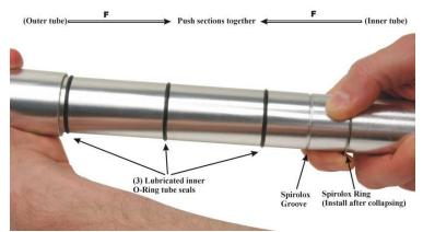
Then install the spirolox around the smaller diameter front tube and position it by sliding it up against the end the end of the larger outer tube.
