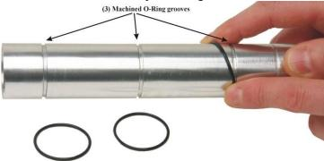
13. Fit inner and outer tube sections together taking care not to pinch or damage any of the pipe sealing rings & collapse completely.
