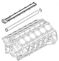
The original bonded seal fails primarily due to corrosion caused by an electro chemical reaction between the materials over time.
