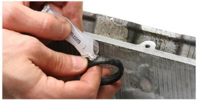
10. Fully fit front seal into housing taking care to make sure the \*flat profile of the seal faces the timing cover (forward). (\*this is critical to a proper installation).
