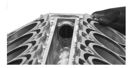
11. Perform the same lubricating and fitting operation to the rear o-ring; noting however there is no orientation necessary for this seal.
