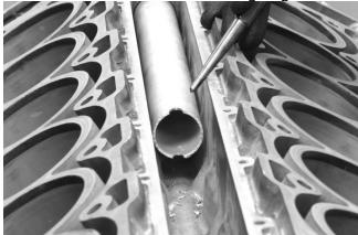
6. Remove the factory pipe in 2 pieces. The front will require some twisting or careful prying to break the bond of the front seal, large pliers are best suited for this job.
