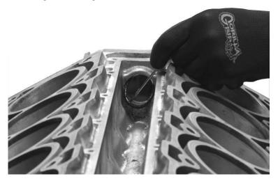
9. Carefully clean the front seal gallery. Lubricate all surfaces of the front seal liberally with the grease provided in the kit.
